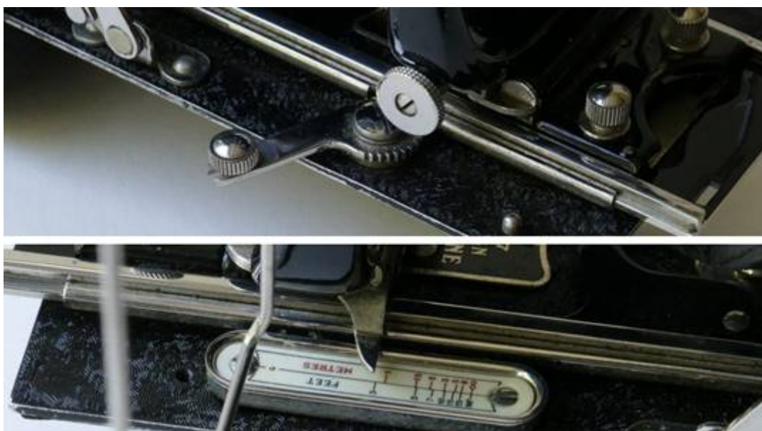
Camera focus ratchet and scale (from 3 feet to infinity)
